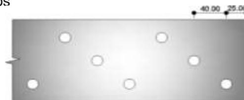
$$Rn2 = (4\text{cm} - (1/2\text{plg} + 1/16\text{plg})/2) * 2.54\text{cm}/1\text{plg}) * (1/4\text{plg} * 2.54\text{cm}/1\text{plg}) * 4570\text{kg}/\text{cm}^2$$
